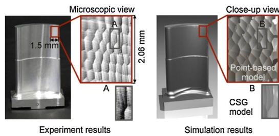
Fig. 12. Measured and simulated surfaces with chatter [44].
