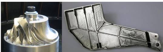
Fig. 2. Examples of machining of titanium impellers.
