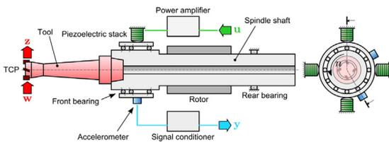
Fig. 32. Active spindle [209].
