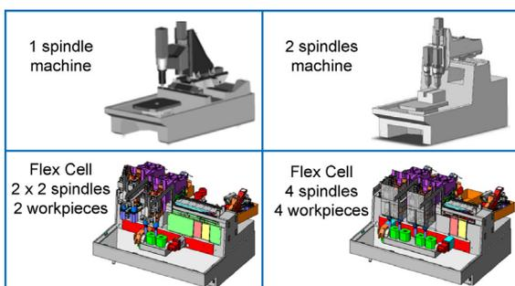
Fig. 13. Machine tool concepts for parallel milling.
