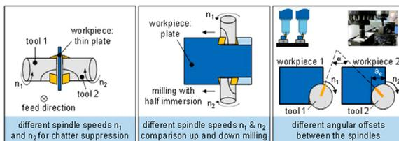
Fig. 29. Chatter suppression for parallel milling processes.
