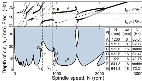
Fig. 26. Iterative procedure for discrete spindle speed tuning.
