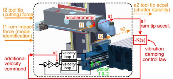
Fig. 30. Active chatter suppression using machine drives [213].
