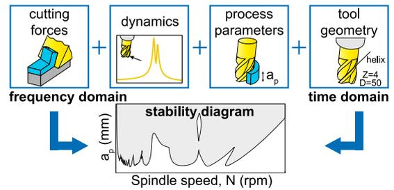
Fig. 5. Procedure to obtain stability lobe diagrams (SLD).
