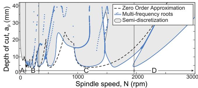
**Fig. 8.** Comparison between different stability models [218].
