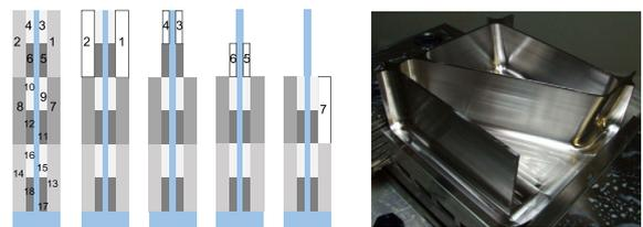
Fig. 22. Waterfall strategy for thin wall machining [192].
