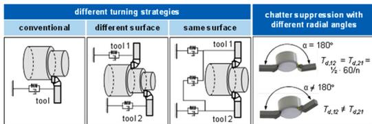
Fig. 19. Chatter suppression for parallel turning [50].
