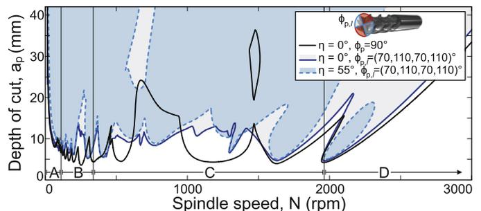
Fig. 16. Effect of variable pitch on SLD.
