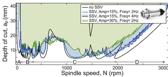
Fig. 28. Effect of SSV in the stability.
