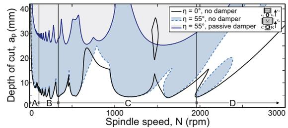
**Fig. 24.** Effect of TMD in the stability.
