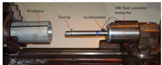
Fig. 31. Boring bar with magnetorheological (MR) fluid [198].
