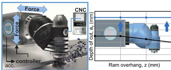
Fig. 34. Dynamic Active Stabilizer (DAS<sup>®</sup>) by SORALUCE.
