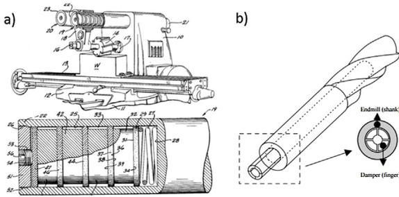
Fig. 25. Friction/impact dampers: [228,356].
