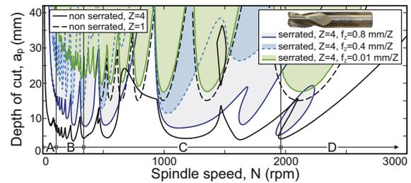
Fig. 17. Effect of the serrated edges on SLD.
