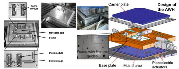
Fig. 33. Active workpiece holder [4,54].
