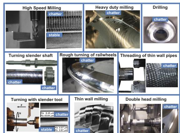
Fig. 1. Chatter problem in numerous machining applications.
