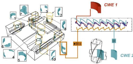
Fig. 6. Tool engagement calculation from CAM model [199].
